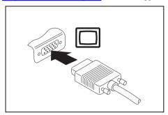
Analogue VGA monitor connection socket
