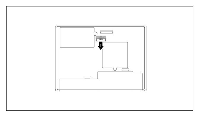
▶ Slide the cover for the battery connector in the direction of the arrow (1).
