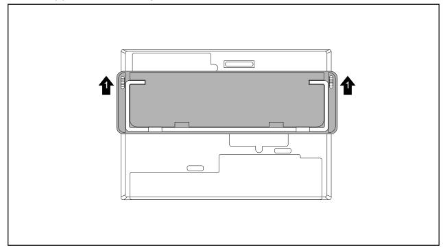
▶ Unfold the tilting device (1) on the battery, if present.
