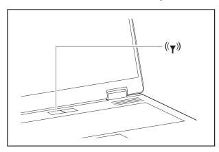
► Press the EasyLaunch button to start the *WirelessSelector*.
