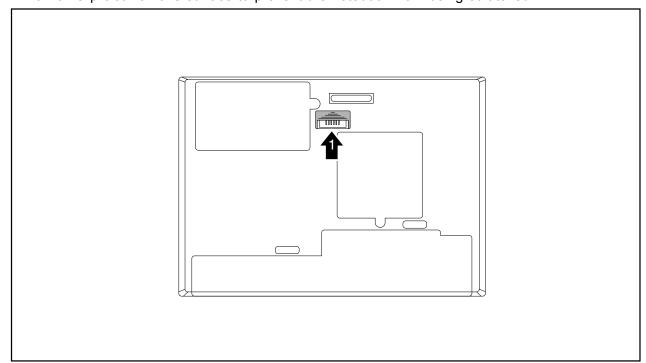
▶ Slide the cover for the battery connector in the direction of the arrow (1).
