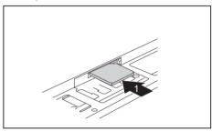
Slide the SIM card into the slot (1) until it is felt to engage, as shown in the battery compartment.
