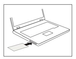
Push the SmartCard into the SmartCard reader with the chip facing downward.
