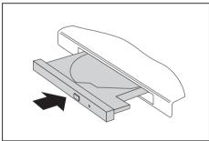
► Place the data carrier in the drive tray with the printed side facing upwards.
