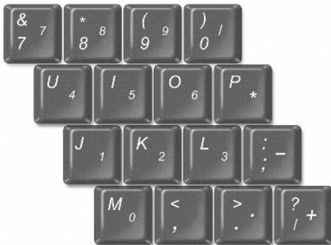
The numeric keypad functions like the numeric keypad on an external keyboard. Each key on the keypad has multiple functions.
