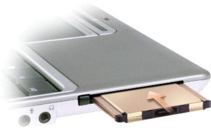
The computer recognizes most PC Cards and automatically loads the appropriate device driver. If the configuration program tells you to load the manufacturer's drivers, use the floppy disk or CD that came with the PC Card.
