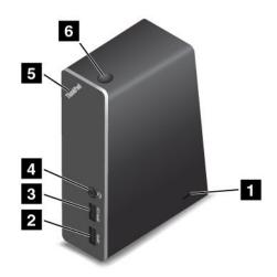
**1** Security-lock slot: To protect your dock from theft, you can purchase a security cable lock, such as a Kensington-style cable lock, that fits this security-lock slot to lock your dock to a desk, table, or other non-permanent fixture.
