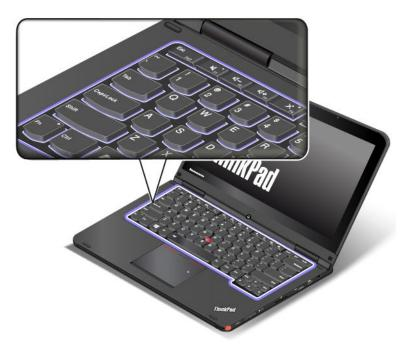
• When you rotate the computer display from 190 degrees to 360 degrees, the frame of the keyboard travels upward for about 2.0 mm (0.08 inch). The following illustration shows the keyboard after the keyboard frame travels upward.
