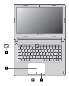
**Touchpad**To move the cursor on the screen, slide your fingertip over the pad in the direction in which you want the cursor to move.
