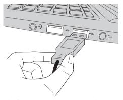
The first time you plug a USB device into a particular USB port on your computer, Windows automatically installs a driver for that device. After the driver is installed, you can disconnect and reconnect the device without performing any additional steps.
