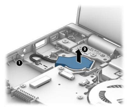
**3.** Remove the RTC battery.
