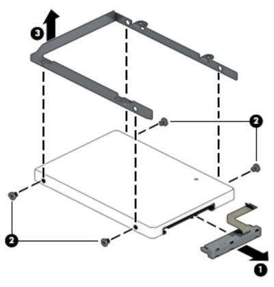
Reverse this procedure to reassemble and install the mass storage device.
