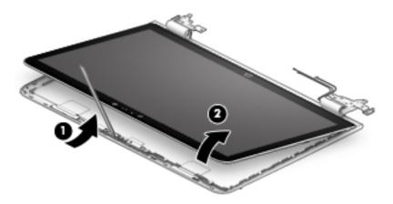
c. Remove the display panel assembly.
