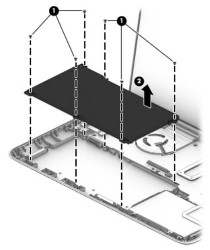
Reverse this procedure to install the battery.
