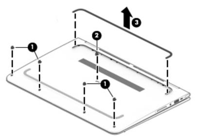
4. Remove the five Phillips PM2.0×5.0 screws (1) and the five Phillips PM2.4×5.7 screws (2) that secure the keyboard/top cover to the base enclosure.
