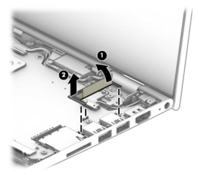
Reverse this procedure to install the USB port shield.
