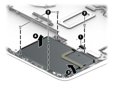
Reverse this procedure to install the mass storage device.
