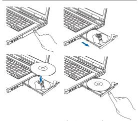
Figure 4-3. Loading/Ejecting Media
