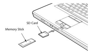
Figure 4-5. Inserting a Memory Stick/SD Card
