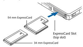
Figure 4-7. Inserting/Removing ExpressCards
