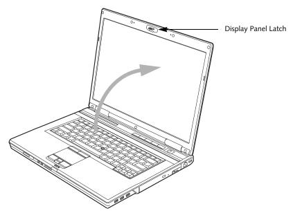
Figure 3-2 Opening the Display Panel
