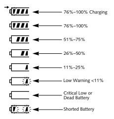
Figure 2-9 Battery Level Indicator
