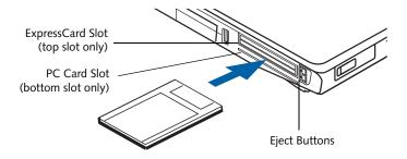
Figure 4-6. Inserting/Removing PC Card
