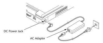
Figure 3-1 Connecting the AC Adapter
