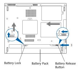
Figure 4-1. Removing a Battery
