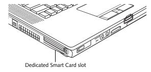
Figure 4-8. Smart Card Slot
