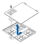
Figure 4-9. Opening the Memory Upgrade Compartment
