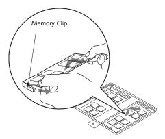
Figure 4-11. Removing a Memory Upgrade Module
