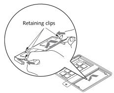
Figure 4-10. Installing a Second Memory Module
