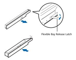
Figure 2-18 Removing/Installing a device in the Flexible Bay
