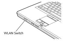
Figure A-3. Wireless LAN On/Off Switch
