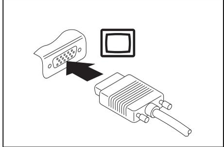
Analogue VGA monitor port (on the device and on the optional Port Replicator)
