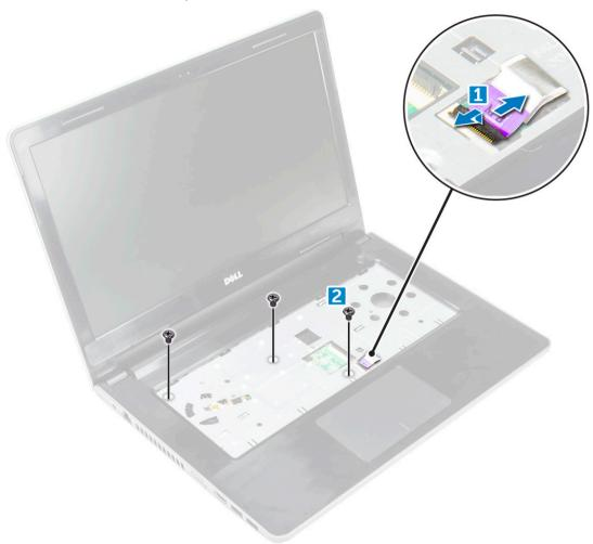
Remove the screws that secure the base cover to the computer
