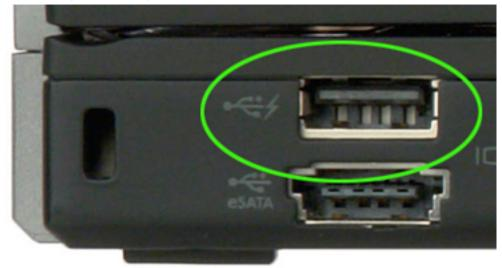
Only the USB connector with a lightning bolt icon, as seen in the image above, can be used.
